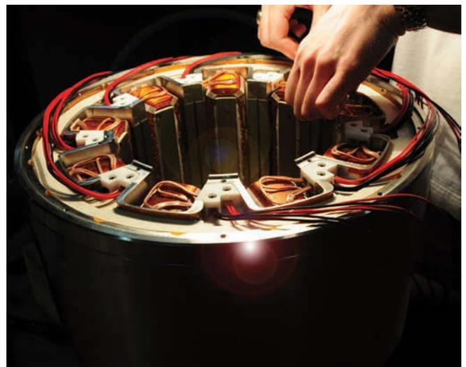
*Final wiring of multi-sector, radial AMB stator*
